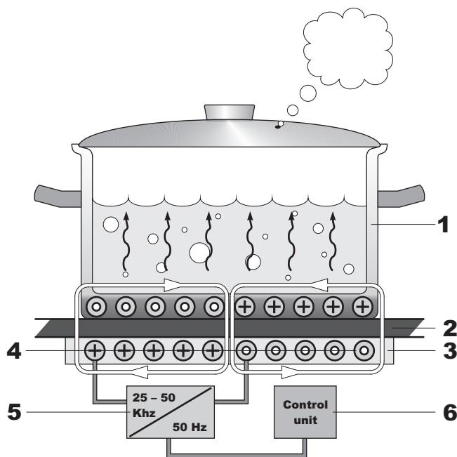
1. Utensil made of ferromagnetic material
