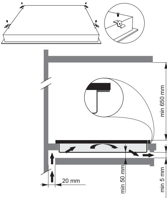
The appliance can be fitted into a working area as illustrated on the figure.
